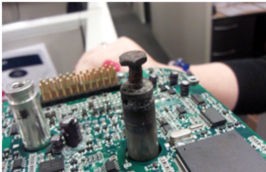
Figure 14: Damaged Controller lug from loose connection. (Case removed for clarity)
